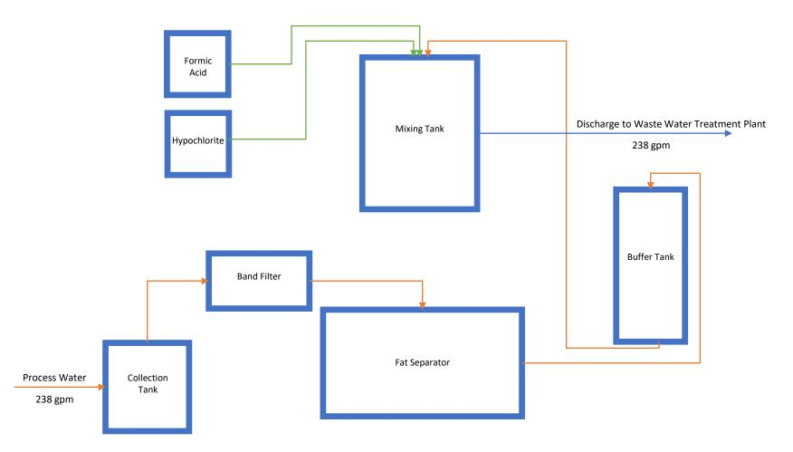
Water used during fish processing originates from the municipal Belfast Water District supply. Wastewater generated undergoes initial disinfection and filtering prior to travelling to the Wastewater Treatment Plant. At the Wastewater Treatment Plant, fish processing water is blended with smolt and grow-out facility production water and undergoes full chemical and biological treatment prior to discharge into Belfast Bay.
