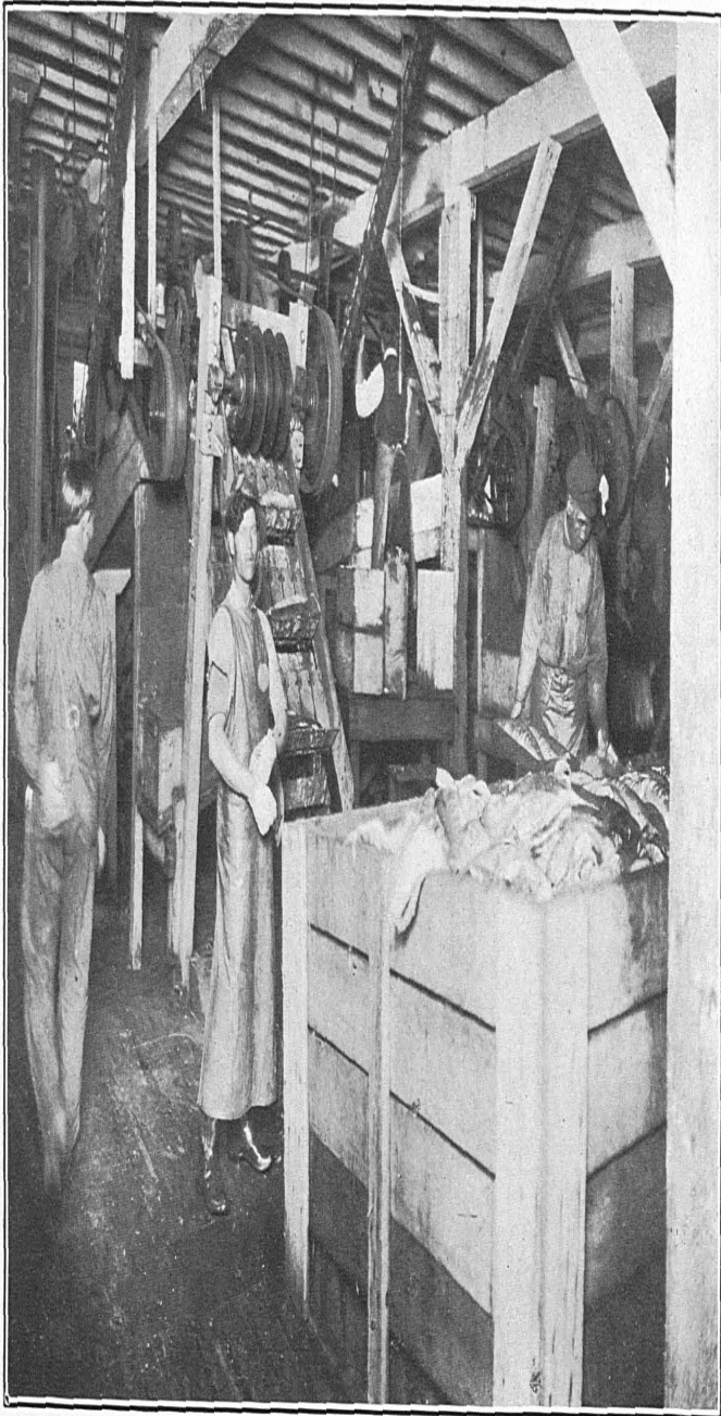
FIG. 29.—CUTTING SALMON INTO PIECES OF A SIZE TO FIT THE CAN.
