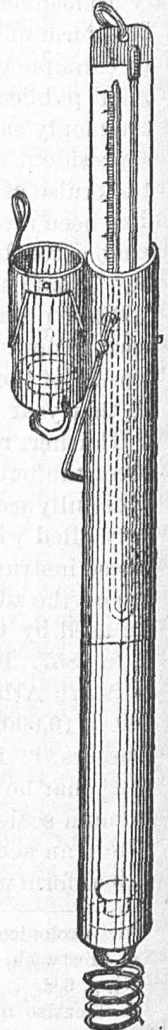
FIG. 7.—Negretti-Zambra self-registering minimum deep-sea thermometer.
