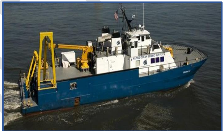
Figure 1 - R/V Shearwater Length 110 ft, beam 39 ft, draft 7 ft
