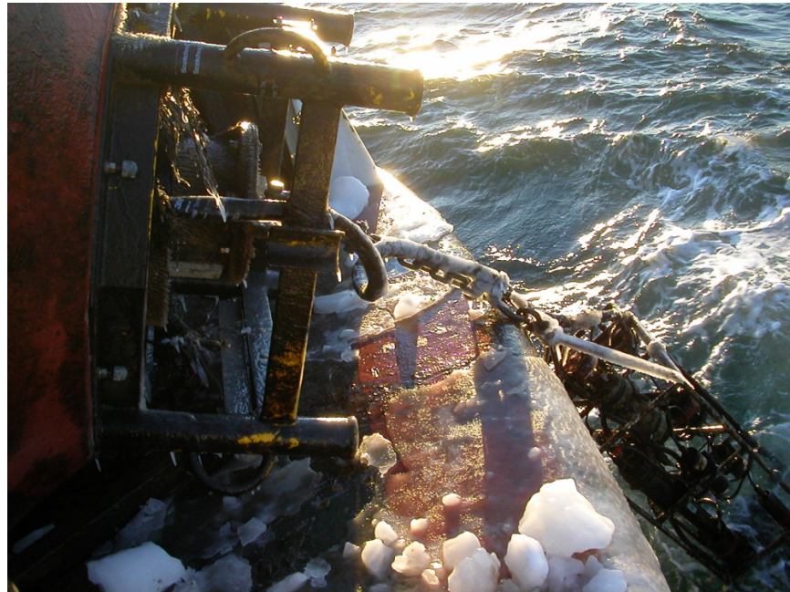
Figure 3-5: Buoy E01 winter ice build-up (January 2004)
