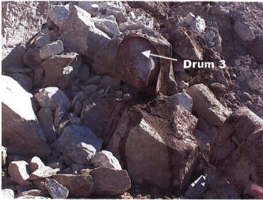
Photo 3 – Drum 3 was partially crushed during the excavation. Oily residue was spilled on rocks and surrounding soil. Environmental Projects tested residue from the drum for chlorinated compounds using a chlor-d-tect kit. Dragon collected a composite soil sample and Maine Environmental Laboratory completed an analysis of the sample.
