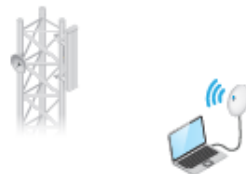
The NanoBeam 5AC Gen 2 as a powerful wireless client.
