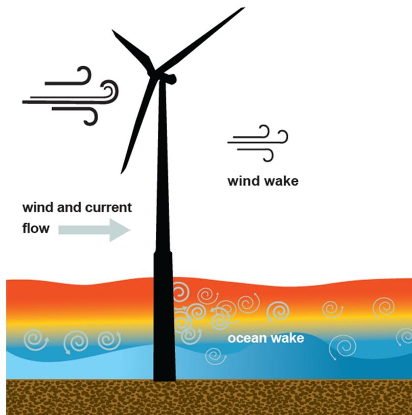
**FIGURE S.3** Schematic of the effects of an individual turbine on local hydrodynamics.
