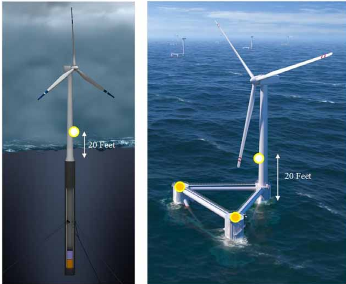
Figure 3-17. Lighting Proposal for Spar (or TLP) Type Platform (left) and Semi-Submersible Platform (right)
